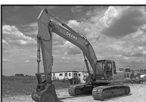
DR4662 '03 John Deere 330C LC excavator
